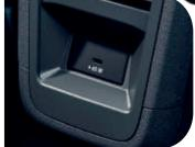
Front & rear fast charge C type 45W
